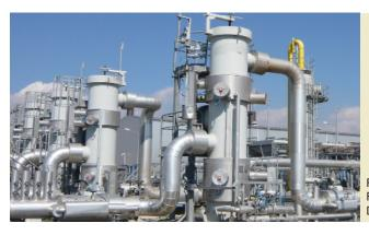
Filter-Separator: Flow rate:491.000 m³n/h Design pressure: 84 bar
